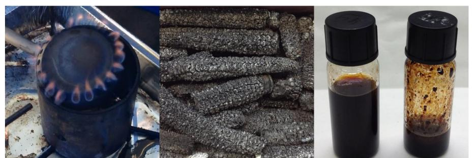
Fig. 4 Valuable products obtained from the prototype TLUD-Pyro stove: syngas, biochar, and bio-oil (from left to right).
