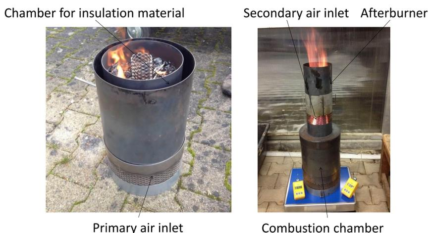
Fig. 1 TLUD stove prototype assembled at Universität Hohenheim.
